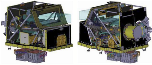
Figure 7: The MSI on-board the Sentinel-2 mission
